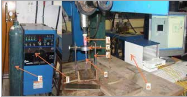
Fig. 1 - Experimental setup: (a) Data acquisition unit (b) GTAW torch (c) Specimen (d) Test rig (e) Thermocouples (f) Power source (g) Shielding gas
